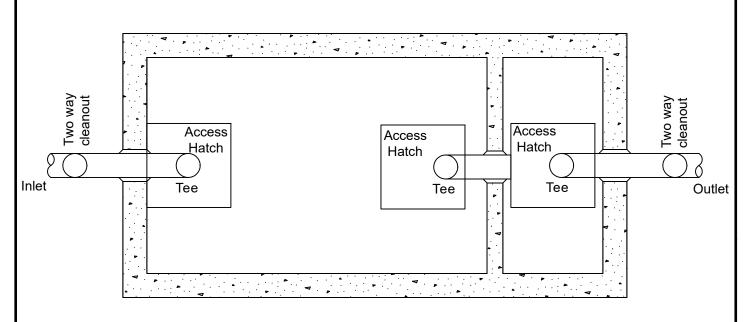
Inside piping, except cleanouts, shall be 4" diameter (minimum)
